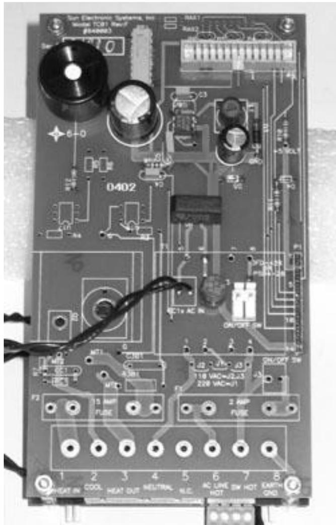
**Fig. 1.4-10 EC0x Rev. F, Power Supply Board**
