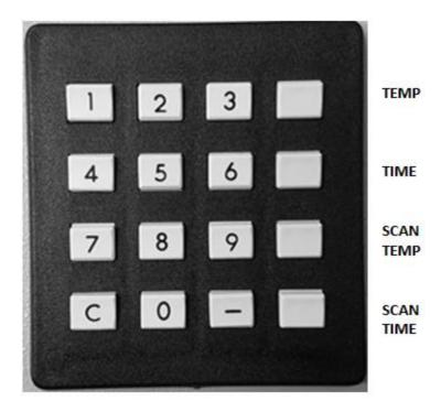
Fig. 3.5-1 Chamber Keyboard Layout 1 (Before 2017)
