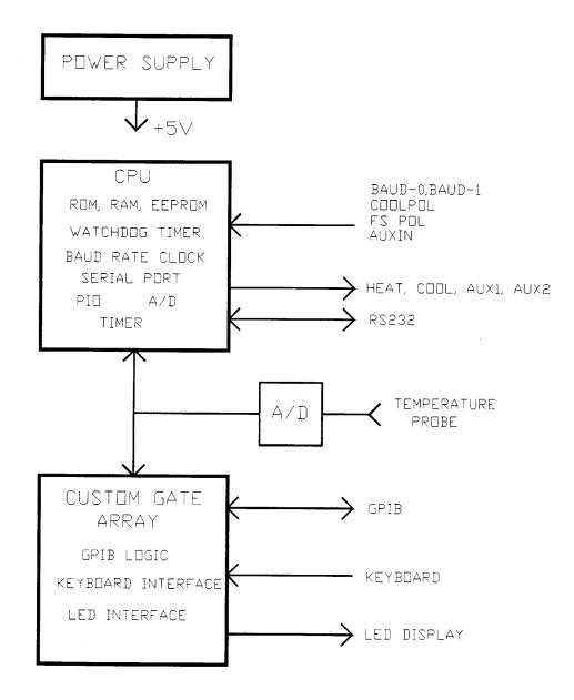
FIGURE 1 TCO1 BLOCK DIAGRAM
