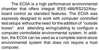
Features of the EC0A include a 0.37 cubic foot working volume, 1200 Watt heating, LCO<sub>2</sub> cooling (LN<sub>2</sub> optional), and a -100°C to +300°C temperature range.
