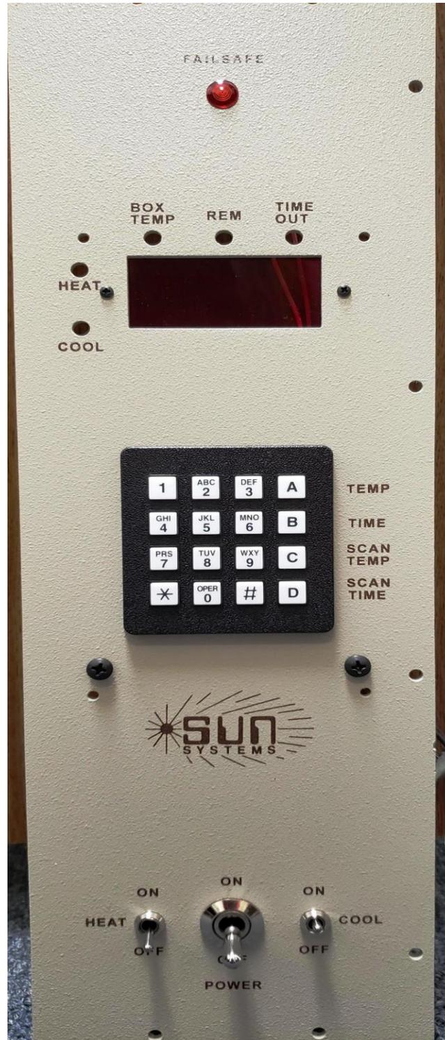
Fig. 1.4-7 EC0x Controller Front Panel
