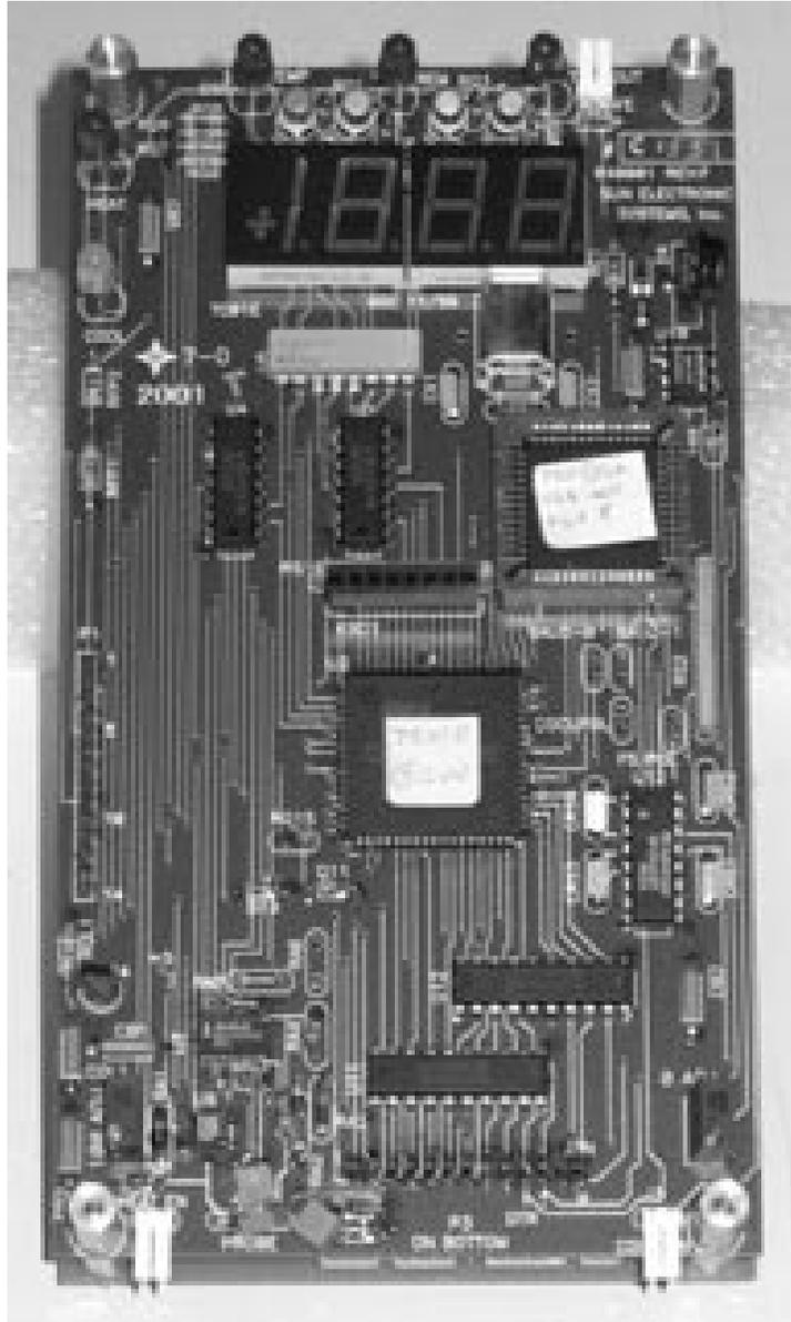
**FIGURE 10 - TC01-F, POWER SUPPLY BOARD**
